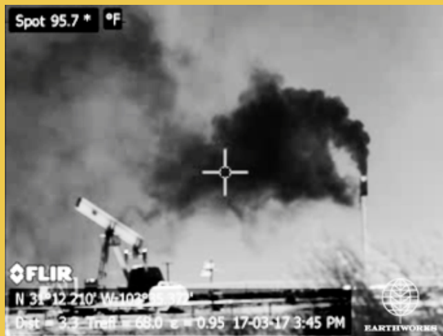
An infrared camera shows an unlit, "venting" flare at an oil and gas production site spewing methane and other pollutants into the air. (Photo credit: Sharon Wilson, Earthworks)
